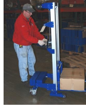
Lower the forks by turning the winch handle counter-clockwise until the load is a few inches above the adjustable leg. Rotate the handle clockwise 1/4 turn to set the winch brake.
