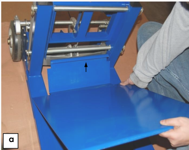
Slide the curved lip of the deck under the lower carriage cross bar.
