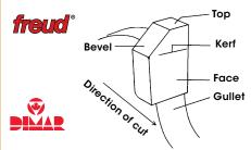
Teeth can have a single bevel, two bevels or no bevel at all. Types of bevels can alternate from tooth to tooth on a given blade. The bevel is what gives the blade its specific cutting pattern.
