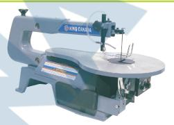
Model No. TBM421 KC-163SSC-V Mfg. No. Capacity: 16" Maximum thickness: 2" Blade length: Speed: Variable (400-1500 SPM) Motor: 1.5 A, 1 phase, 60 Hz Voltage: 110 V Dimensions: 25" L x 13" W x 12 1/2" H Weight: 42 lbs. Price/Each Ś
