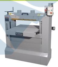
Model No. WK980 Mfg. No. KC-26DS 3 HP 220 V, 1 phase Drum motor: 1/4 HP, 220 V, 1 phase Belt feed motor: Maximum width of sanding: 26" Maximum thickness of board: 12" Minimum thickness of board: 1/4" Minimum board length: 5" Feeding speed: 3-20 SFPM Number of sanding drums: Drum speed: 1600 RPM Voltage: 220 V, 1 phase, 60 Hz 45" L x 30 1/2" W x 49" H **Dimensions:** Weiaht: 485 lbs. Price/Each Ś
