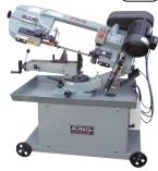
**TBU410** Model No. Mfg. No. KC-712DS Cutting capacity at 90°: Rect. 7" x 12", Round 7" Rect. 3-1/2" x 5-1/2", Round 5" Cutting capacity at 45°: Speeds: 4 (98, 164, 246, 328 FPM) 0.75" x 0.032" x 93" Blade: 1 HP, 6.2 A, 1 phase, 60 Hz Motor: Voltage: 220 V **Dimensions:** 50" L x 26" W x 44" H 325 lbs. Weight: Price/Each
