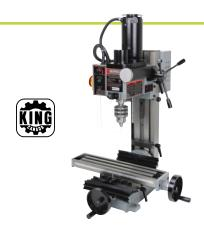
UAD693 Model No. Mfg. No. KC-15VS Drilling Capacity: 1/2" Max. distance spindle 11-1/4"" nose to table: Speeds: Face mill capacity: 1-1/8" End mill capacity: 5/8" Working area of the table: 3-5/8" x 15-3/4" Size of T-slot on table: 7/16" **Dimensions:** 19-1/2" x 22" x 30" Price/Each
